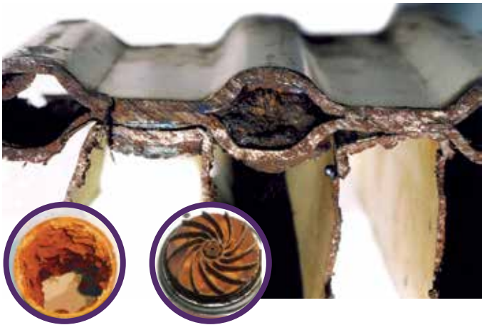
Damaged installation components due to water contamination
